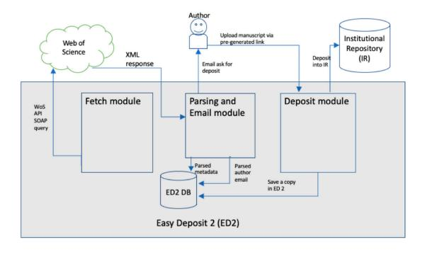
Figure 1. Easy Deposit 2 (ED2) system diagram.
